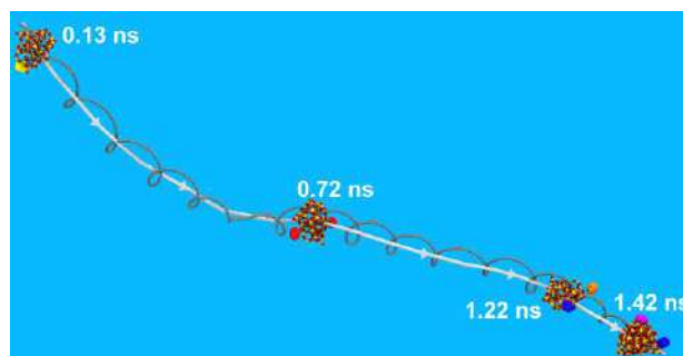
Figure 1. The trajectory of a 1.5 nm silica NP (in red and yellow bonds) diffusing in air with snapshots at 0.13, 0.72, 1.22 and 1.42 ns with colliding gas molecules (yellow, red, blue, and orange dumbbells).
