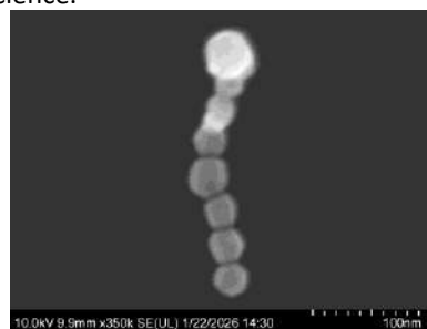
Figure 1. SEM image of the Pt 2 FeNi nanoparticles. This work was supported by the Wallenberg Initiative Materials Science for Sustainability (WISE) and NanoLund.
