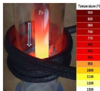
Figure 2. Picture of the inductive coil, the glass tube, and a heated iron workpiece of the heating generator operating with N 2 as the quenching gas.
