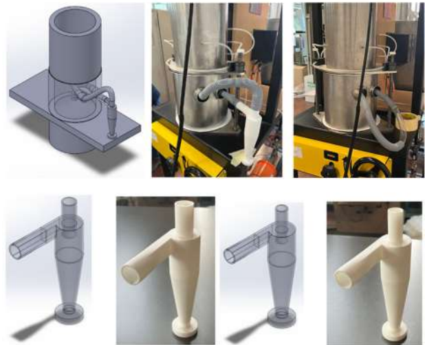
Figure 1. Cyclones produced by additive manufacturing (bottom) and test rig for measuring their performance.
