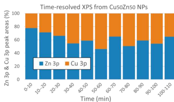
Figure 1. Indication of the relative amount of Zn and Cu on the NPs surface over time, captured by in-flight XPS. The NPs were generated using Cu 50 Zn 50 alloys.
